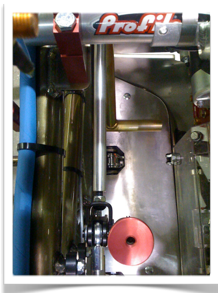
TOP VEIW FRAME, MASTER CYLINDER RODS BRAKE ROD ALL RUNNING PARALLEL
